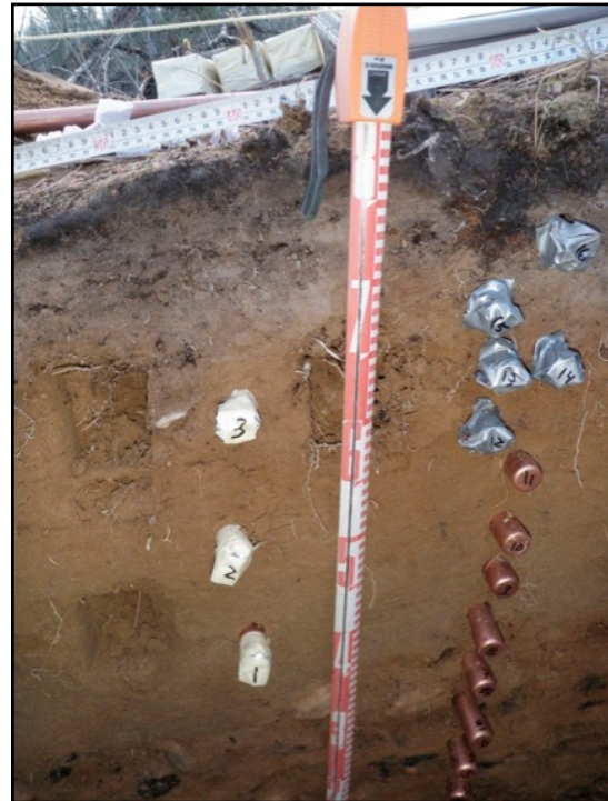
Figure 1. Samples placed for optical profiling (right) and formal optical dating (left) in a typical northern Alberta sediment profile on an archaeological site.
